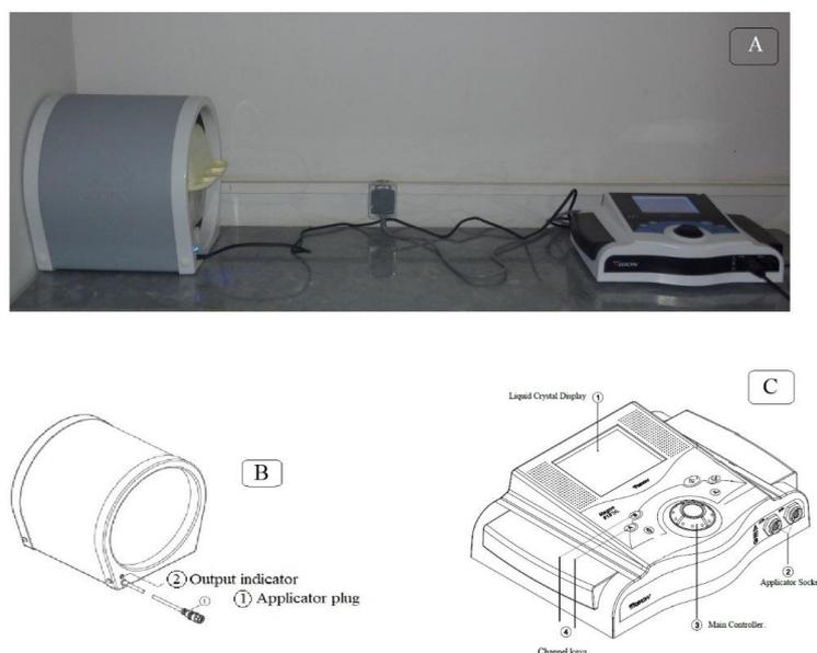
**Figure 2.** A: Electromagnet generator device (Model Magno 915X, Novin Medical Engineering Company, IRAN). B: solenoid coil C: regulator
