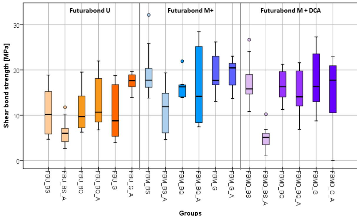
**Figure 4.** Boxplot showing SBS with the corresponding groups without (25) and after the aging process (marked with an “A” in the group name) plotted next to each other (e.g. FBU\_BS vs. FBU\_BS\_A)
