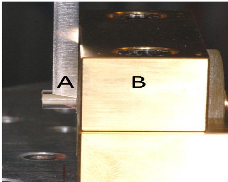
**Figure 3.** Photograph of the fixation jig (B) and the positioned blade edge (A) before Shear-bond tests
