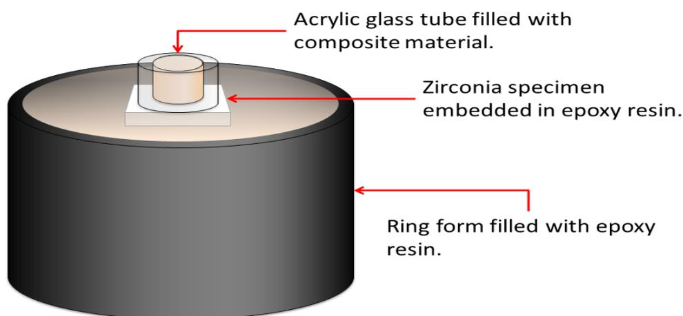
**Figure 1.** Schematic drawing of the specimen design.
