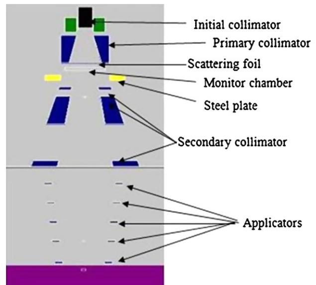
Fig. 2 – Schematic design of Neptun's simulated components.
