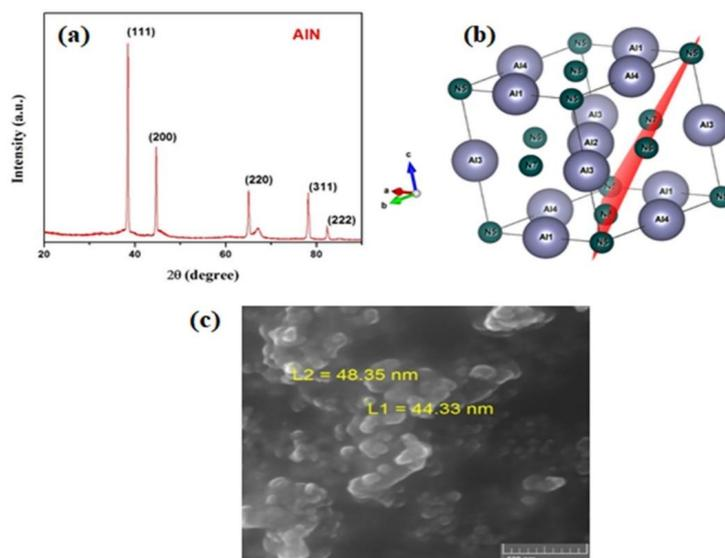
Fig 1. a) XRD Pattern of Synthesized Sample, b) Cubic Structure of AlN Nanoparticles Generated Using VESTA Software, c) FE-SEM Image of AlN Nanoparticles
