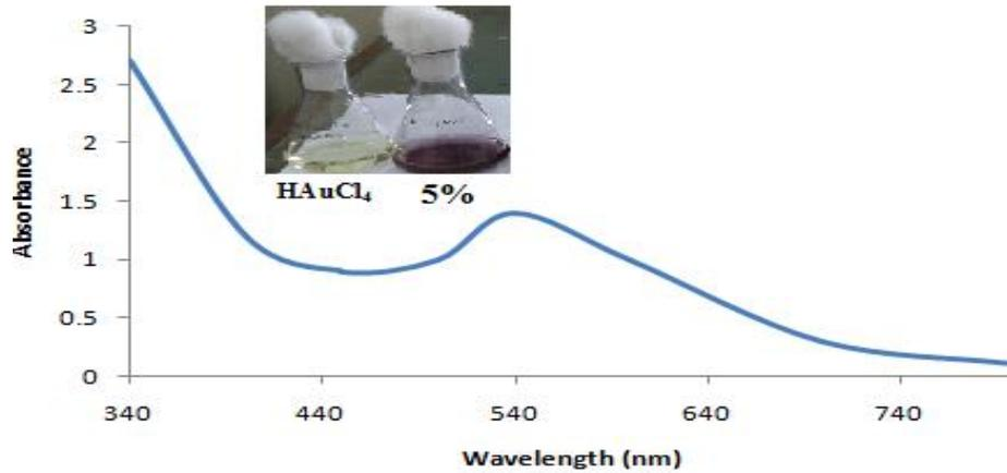
**Figure 1.** UV-vis-absorption spectra of 5% methanol extract phytochemically synthesized gold nanoparticles. The inset image shows the 1mM HAuCl<sub>4</sub> solution and green synthesized gold nanoparticles solution.
